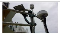
**Comment from PI:** The meteorological station is mounted at the top of the BOREL superstructure. There is no central data storage available on the buoy.
