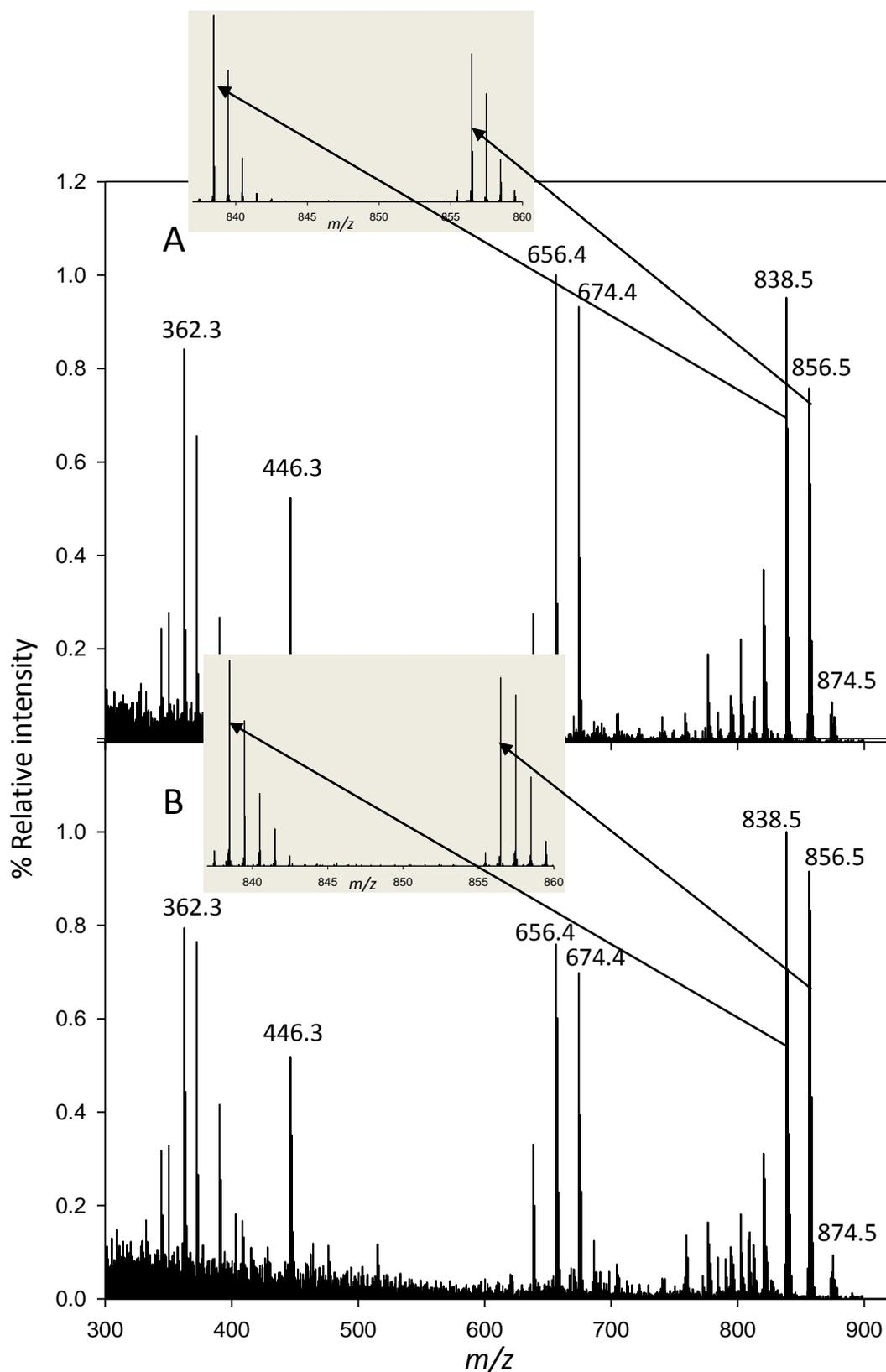
**Figure S4.** Mass spectra of A) AZA15 following heating of hepatopancreas extract in MeOH and B) AZA15 showing incorporation of deuterium (increase in isotope peaks) following heating of hepatopancreas extract in  $\text{CH}_3\text{OD}$ .
