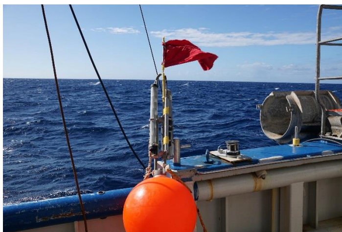
Figure 7. Main buoy with radio and GPS beacon attached.
