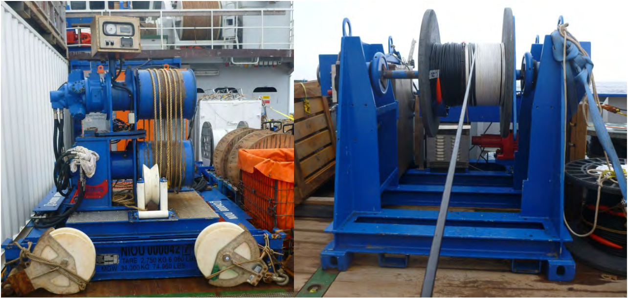
Figure 3: a) The NIOZ LEBUS Double Barrel Winch, b) the spooling winch used with the DB winch. Photo's: Colin Griffiths.
