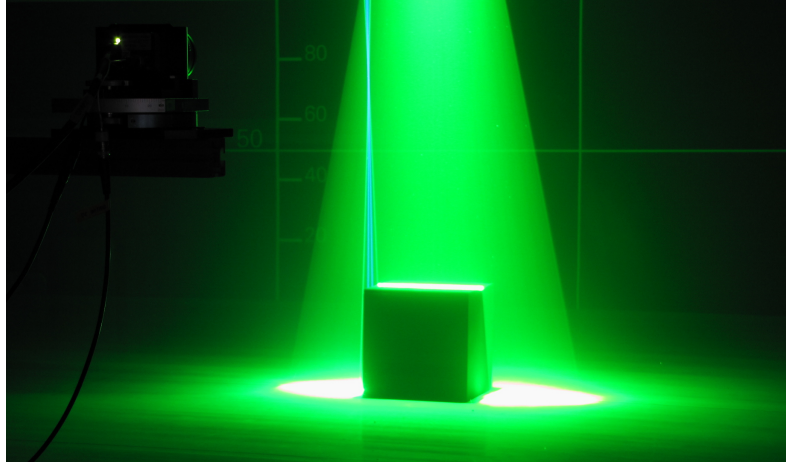
Figure 2 – Cube during simultaneous PIV and LDV measurements, flow coming from the left.
