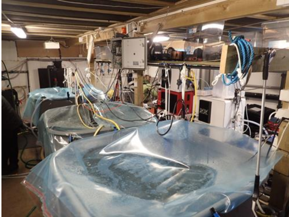
1 Three 1 m 3 water tanks coated with plastic foil in order to minimize the effect of atmosphere-water exchange
