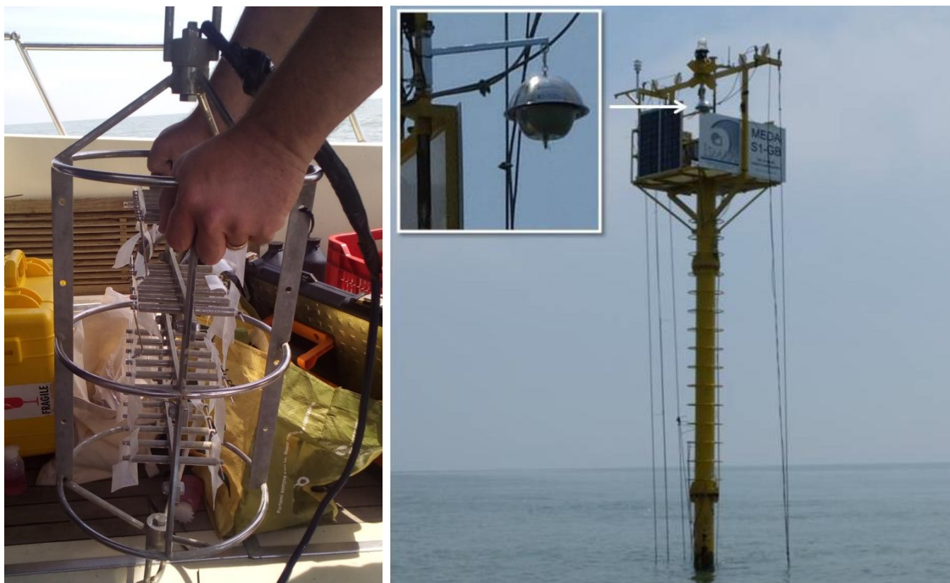
Figure 4: Mounting the sampler sheets (left) and deployment aquatic and air passive sampler (right)
