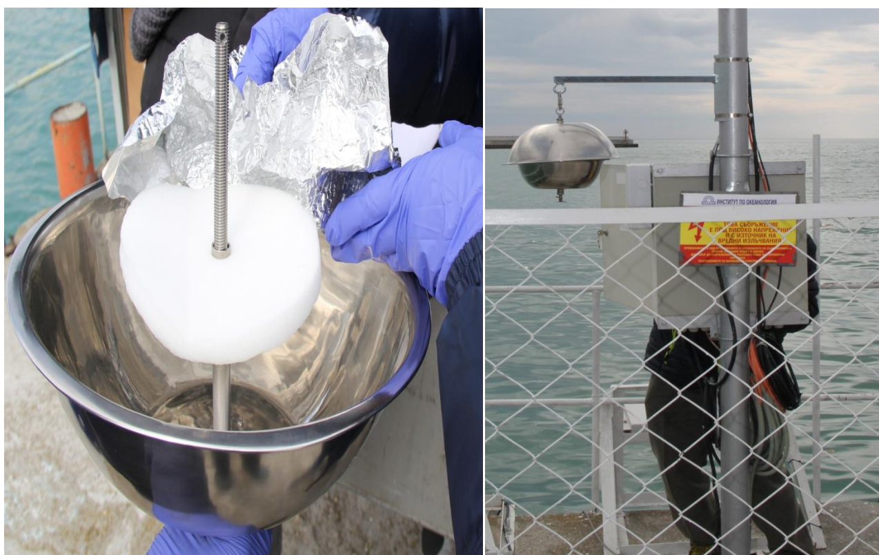
Figure 2: Place the PUF disk (left) and deployment air sampler (about 2 meters above ground) (right)
