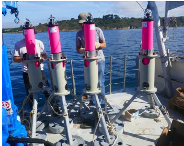
Figure 2 : The 4 Canopus acoustic beacons in their fancy pink sleeves, mounted on tripods.
