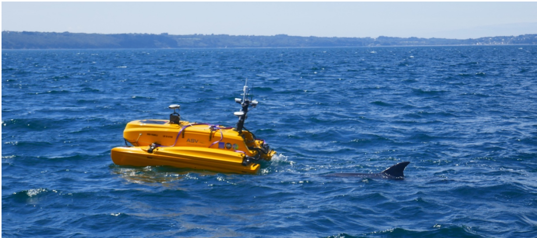
Figure 4 : The USV (named PAMELI) of the LIENSs laboratory in la Rochelle in action, followed by an intrigued visitor. The USV is a 3m-long over 1.6m-wide catamaran, weights 300kg, and is battery powered (8h autonomy).
